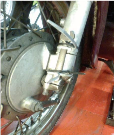
for hours waiting for a recovery vehicle, I rigged up a splint from a spanner and some cable clips to add support to the spring rod inside the fork leg. Knowing that it wouldn't come apart, I rode the Crusader home at a gentle pace, doing all braking at the rear wheel.
