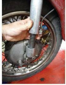
for hours waiting for a recovery vehicle, I rigged up a splint from a spanner and some cable clips to add support to the spring rod inside the fork leg. Knowing that it wouldn't come apart, I rode the Crusader home at a gentle pace, doing all braking at the rear wheel.
