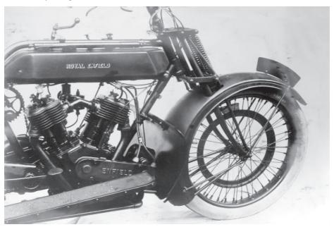
In general design, as will be gathered from the photograph, the machines are standard, the new type of fork with double spiral spring in front being, of course, used. The Palmer Cord tyres on the machines are 700x 80 mm section. The mudguards of the standard Enfield have always been of liberal dimensions and flat, so rendering them suitable for extremely muddy conditions.
