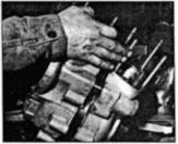
Heat timing side case with outer roller race and drop it over crankshaft. While doing this, make sure to lift the tappets clear of cams.
