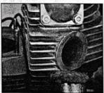
See that dowels are in position in the barrels and push rods are right way up. Coat both sides of copper gasket with compound and slip head on.
