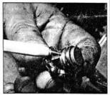
In the older type clutches there is a clutch thrust bearing which should be examined for wear before replacing. Look especially for pitting on track.
