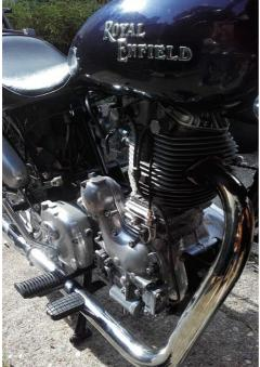
became my everyday go-to machine, bypassing more powerful Japanese multis sulking in the garage. The sprag clutch packed up as expected, so I took the opportunity to remove the starter motor, solenoid and associated wiring so I wasn't carrying any unessential weight. I blanked off the starter motor hole. This bike kickstarts easily enough if you know how to do it!
