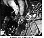
Grease the balls which go between the torque arm and clutch operating lever when front plate is in position. Don't forget washer on bearing.
