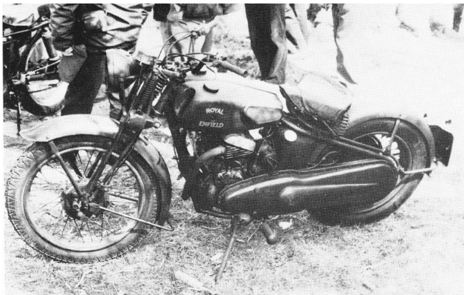
Engine detail shows forward facing carburettor, camshaft cover plate and separate oil tank.
