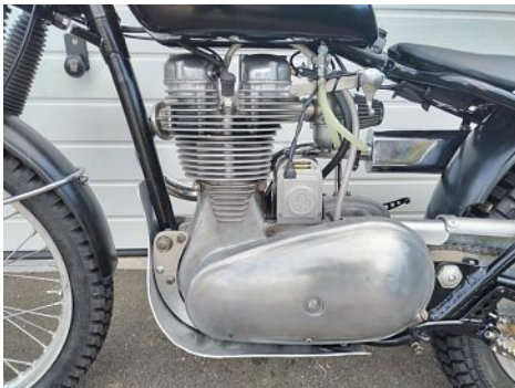
Conspicuous by its absence, the missing gearbox frame brace saved weight and offers clean lines.
