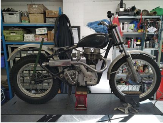
The mock up 'spares pile' variant in October 2022. Excelsior Consort tank, MP forks and cut down RE front hub.
