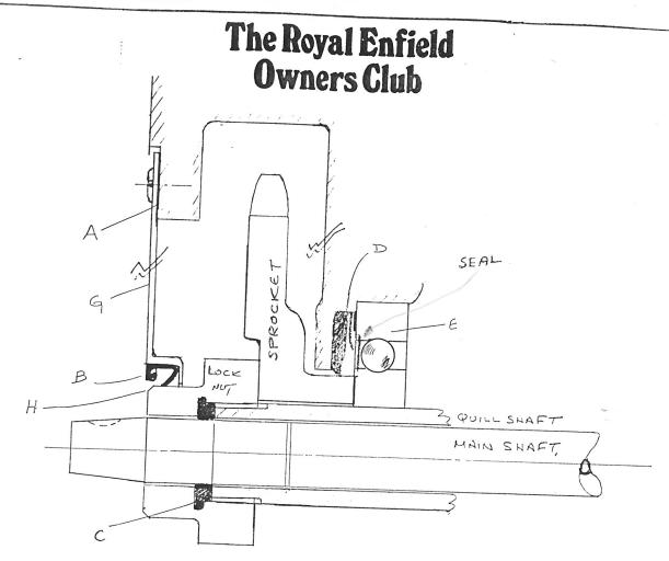
There are a number of seals which, if they fail, leak oil into the rear chain area.
