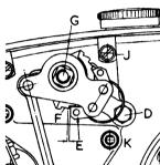
Remove from crankcase the two gearchange stop pegs on either side of gearchange lever. Should there by any oil leakage after removal of these pegs, fit the two smaller diameter pegs supplied. These are quite unnecessary if there is no oil leakage.
