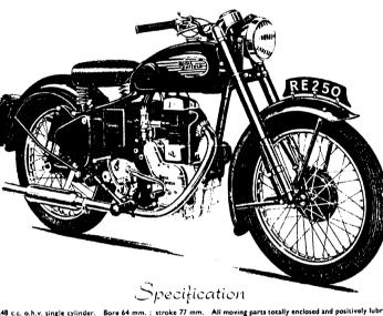
which utilises large capacity oscillating plunger-type feed and return pumps and incorporates a highly efficient felt oil f ted with oil-wetted air filter. GEAR BOX: Four speed foot-operated gearbox. Multi-plate clutch. Ratios, 6-2. ANSMISSION: Primary drive by !" pitch chain totally enclosed and running in aluminium oilbath chaincase. F
