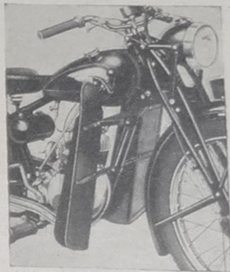
Useful legshields for the rider who must keep clean even in the dirtiest weather are obtainable for the 125 c.c. model
