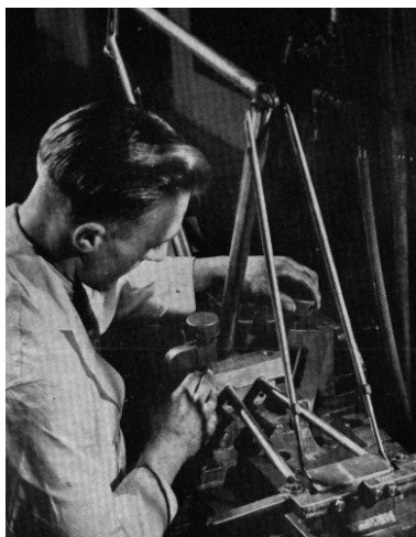
Left: Victor Heath setting up a jig for welding the rear fork tubes to the bottom bracket. Right: One of the welding operations in progress. The "firework" display is quite harmless, as will be vouched for by the operator, Bernard Franklin, assistant foreman.
